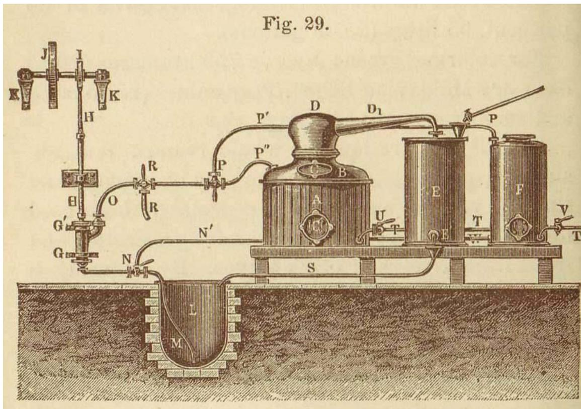
This apparatus performs the different operations in an excellent manner by the use of one pump which charges the still, A, with water, conducts the distillate into the coloring boiler, and the finished product into the barrels. This is done in the following manner:
